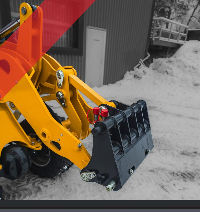
Experience the convenience of our hydraulic quickhitch system, featured prominently in our H280 series. Designed for seamless attachment changes, it enhances operational efficiency. We offer various standard options and customizable configurations. Contact us to explore available options tailored to your specific requirements and region.
