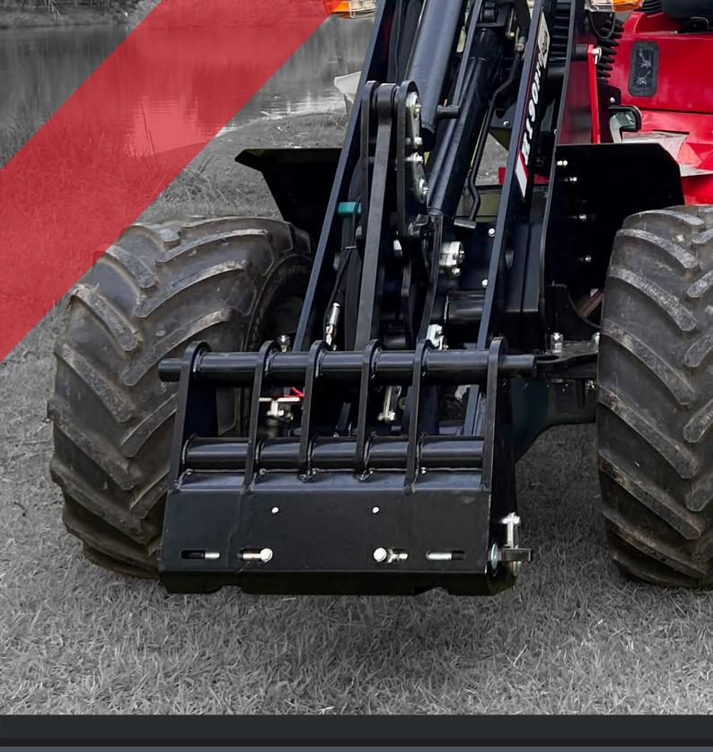
Each H220 model boasts a robust hydraulic quickhitch system with an extensive selection of attachments, ensuring unparalleled versatility across various tasks. From standard configurations to custom options tailored for specific regional needs, our loaders accommodate a wide range of applications. Explore our attachments including buckets, pallet forks, and snow blades, demonstrating the machine's adaptability and efficiency in diverse environments.
