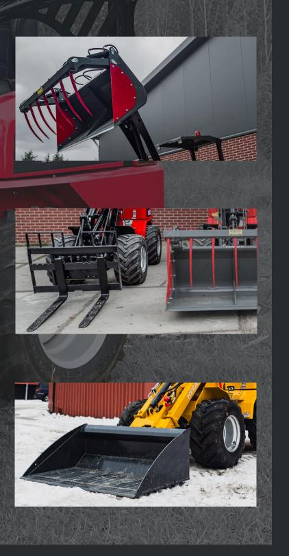
Enhance the versatility of your H190 wheel loader with our wide range of attachments. Choose from essential tools like pallet forks for precise material handling, pitchforks for agricultural tasks, stone buckets for robust material handling, and bale grabbers for efficient hay and straw handling. We offer a variety of options to suit your specific needs and maximize productivity in farming and construction applications.
