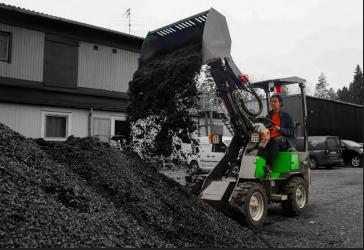
**The H160** sets the standard for agility and performance in compact machines. With its low weight and high steering angle, navigating narrow spaces is effortless. Equipped with the Avant quickhitch as standard, it's perfect for tasks requiring precision and strength. Hydraulic motors on each wheel and optimized hydraulic functions ensure compatibility with a variety of attachments.
